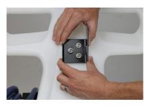
**3b.** Install the nylock nuts to the screw and tighten. You will need to put your arm into the inside of the tank.
