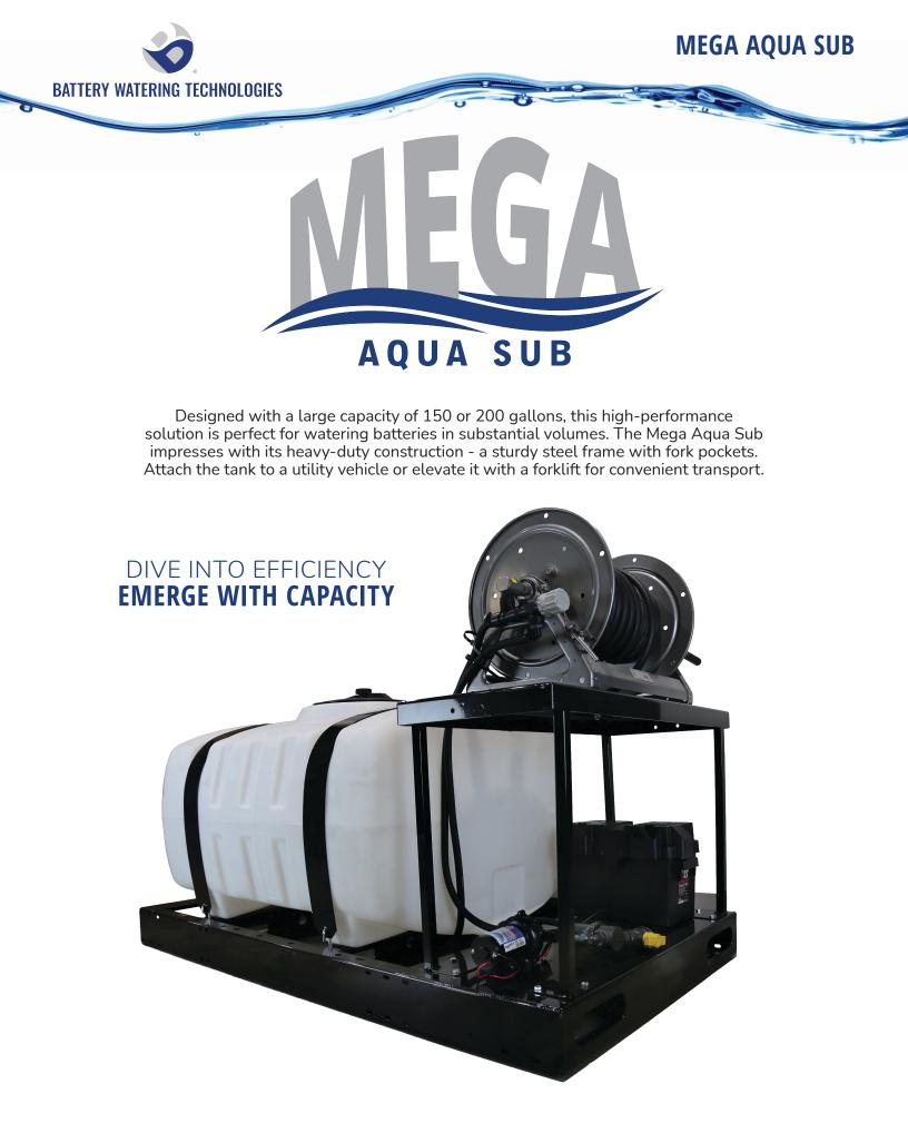
**150 & 200 GAL CAPACITY -** Thick-walled polypropylene tank is corrosion resistant with a large vented screw-top lid for easy filling. The translucent tank with gallon and liter graduations allow for quick visual checks of the water level. For best results, fill tank with deionized water from our Deionizer (Part # PW-1800).
